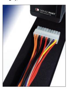
"Is the right cable in the allocated place on the connector?" The FA 45 identifies, sorts and inspects up to 32 taught colours – even "non-colours" such as grey, white, black.
