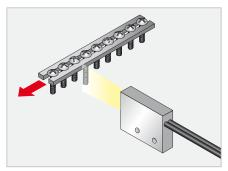
The sensor supplies an analogue signal, which is proportional to the reflectivity of the object being detected and which in turn is proportional to the distance, size, surface, etc, when reflectivity from the object is identical. The FL 70 RA-D sensor enables analogue output of the length of screws.
