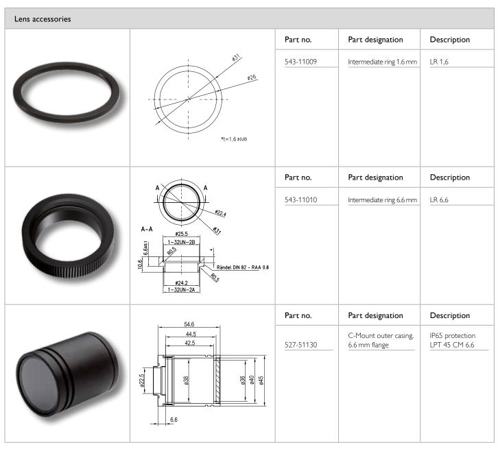
Intermediate rings and outer casing for C-Mount lenses.
