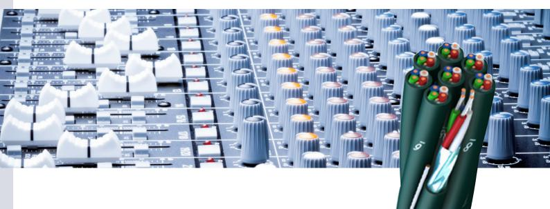
Event 220Series is a Pre-Jacketed starquad audio multicore with individually foil sreened quads and overall foil screen. Each quad jacket is made of a soft LSZH material and the overall sheath is a leading edge LSZH Polyurethane (PUR) material. In the case of the single quad the sheath is the LSZH PUR.
