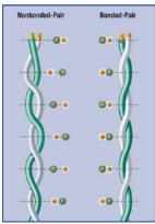
Bonded-Pair cables have a uniform conductor-to-conductor spacing; nonbonded-pair cables are inconsistent.
