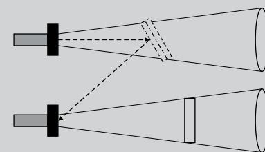
The above-mentioned mounting distances are only intended as a guide. In the case of tilting, the sound can be reflected towards the neighbouring sensor. The minimum distance should then be determined by means of trials. Some sensors permit synchronisation with one another and thus allow considerably lower scanning distances.
