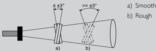
Ultrasonic sensors can be installed and operated in any orientation. Though installation locations that could lead to contamination of the sensor surface should be avoided because water droplets and encrustation can impair functional performance. Thin layers of dust and paint droplets generally have no effect.
