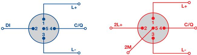
Class A Ports (X1-X4) are best suited for sensors because next to the usual Pin 4 (IO-Link communication) they have an additional hardwired digital input channel on Pin 2. This allows a total of four additional digital inputs.
