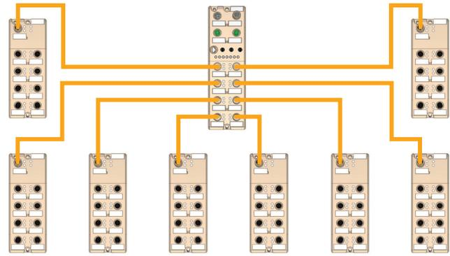
When LioN-Power IO-Link I/O Hubs are combined with the LioN-Power IO-Link Masters, you can **cost-efficiently transmit a maximum of 132 digital signals up to 20 m away from the Masters**. This enables efficient upgrades from passive to active systems, or for distributed environments to collect many digital signals.
