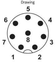
Pin assignment M12-plug, 8-pol, A-coding
