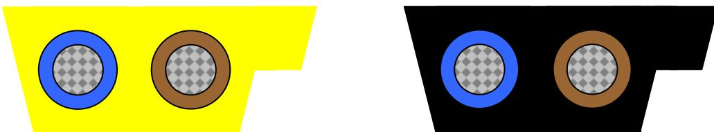
Conductor                    Tinned copper wire, 1.5 mm<sup>2</sup>, finest wire acc. to VDE 0295 class 6
